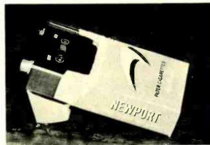
BUGGING TRANSMITTER, concealed in flip-top cigarette pack, has a built-in antenna giving it a range of up to two city blocks.
