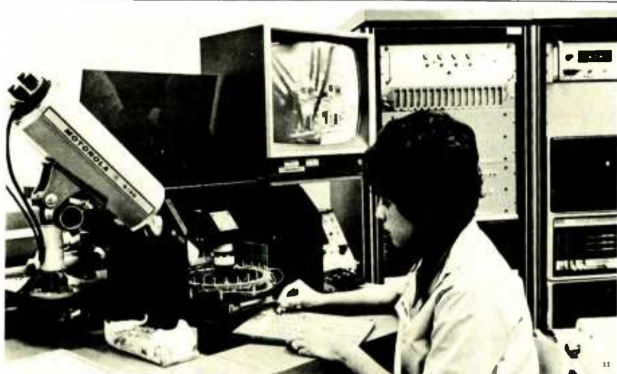
Laser resistor-trimming set-up at Motorola. Resistors on hybrid circuit substrates are trimmed to tight ohmic tolerance by a laser beam which cuts into the film resistors used. The TV monitor displays hybrid circuit workpiece, while the computer/measurement system (on the right) monitors and controls the trimming operations.
