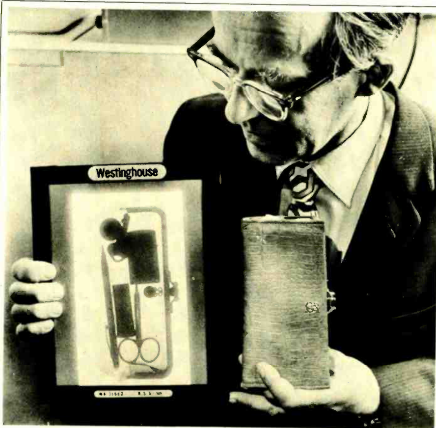
THE CONTENTS OF A LADY'S PURSE show up on a storage-type radiographic amplifier screen.
