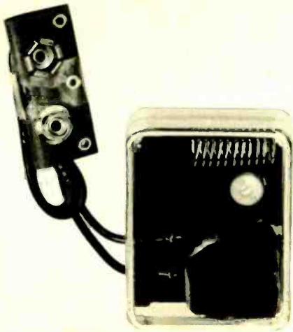
FIG. 1—INEXPENSIVE WIRELESS BUG transmits on an unused portion of the standard FM broadcast band.
